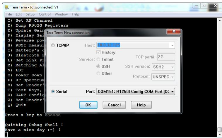
5. Press the "ESC" key to access the reader configuration menu:
