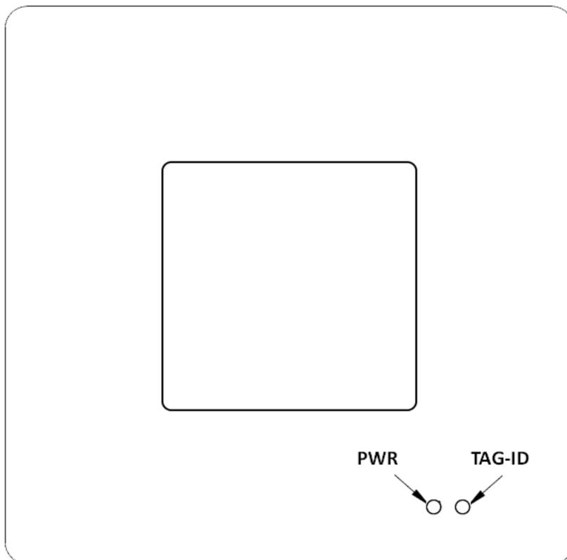
Fig. 1.4: Tile R1251INF Front Panel LEDs
