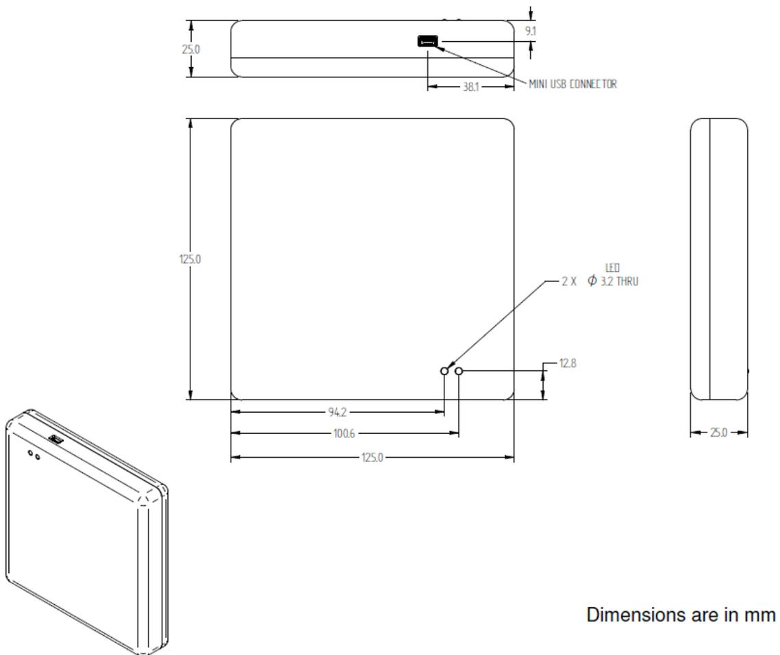
Fig. 1.3: Tile R1251INF (standard enclosure) mechanical drawing
