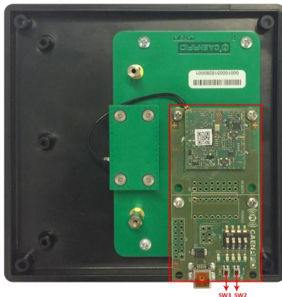
3. Press the reset switch on the evaluation board (SW3).
