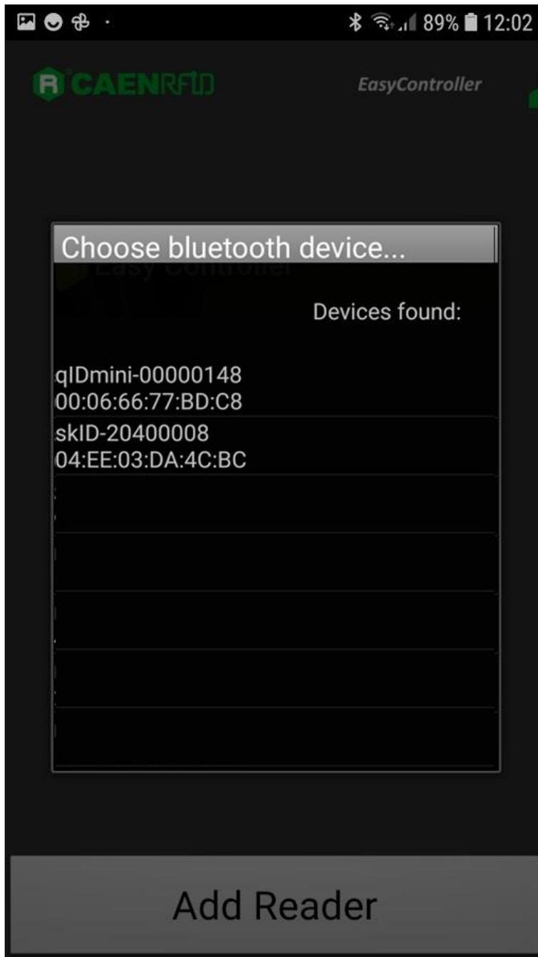
6. Once the connection is established the Bluetooth blue LED of the reader turns on (see § Tab. 1.4: Bluetooth and USB/charger LED status table page 10).
